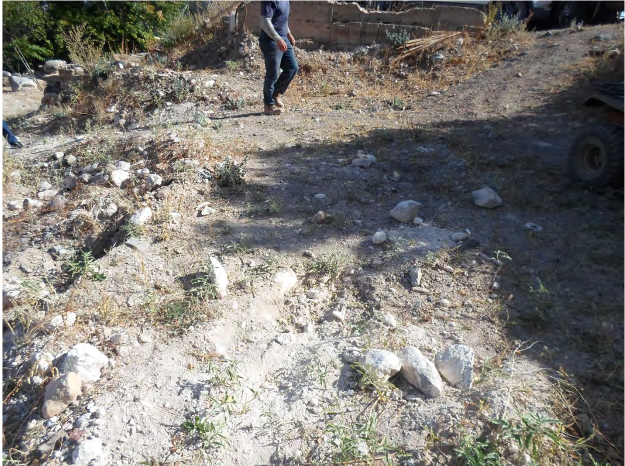
Photo 2 – View looking north across the site at the area of the main residence. The location of Boring 1 is in the foreground. Note the white very dense and strongly cemented clayey sand gravel soils which are exposed on the surface at this location. These soils were not encountered at the location of Boring 2, but likely exist at a depth greater than 2.5 feet at that location.
