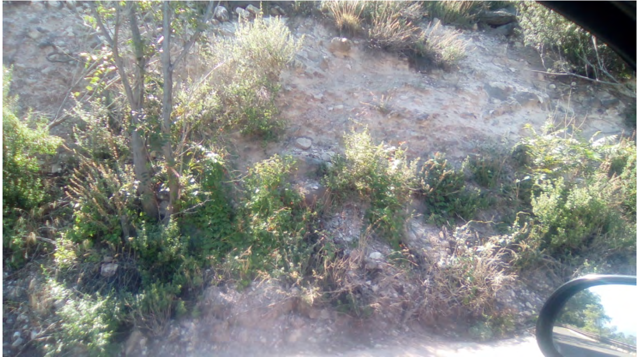
Photo 7 – View looking at a roadway cut below the site of the proposed residence, showing the very dense and strongly cemented clayey sandy gravel that exists below the site. This material was encountered in Boring 1 near the surface, but was not encountered at the location of Boring 2. Foundations should bear on this material.
