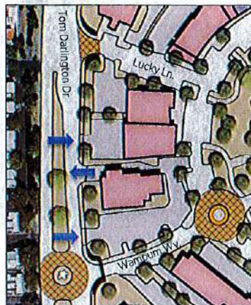
Existing Conditions: Currently there are several entry roads and driveways along Tom Darlington Drive that impeded traffic flow and clutter access to the Village Center.
