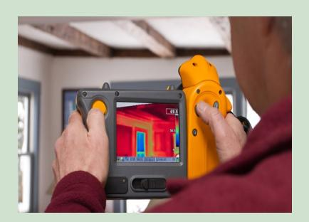
The images can reveal where walls, ceilings or floors are inadequately insulated or where windows and doors aren't well sealed.
