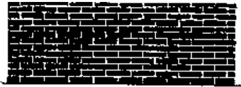
Masonry Wall (poured concrete, stucco, concrete block, brick, etc.)
